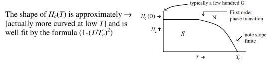
The reason for the existence and behavior of the critical field  $H_c(T)$  is a straightforward thermodynamic one: the *S* state has a negative (condensation) energy relative to the *N* state, but since it excludes the magnetic field entirely, this costs an (extra) energy
