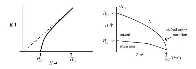
Anticipate: in mixed state, magnetic field punching through in form of vortices (cores effectively normal), while bulk remains superconducting.
