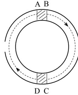
A single junction in a transverse dc magnetic field may be regarded as the continuum version of the above dc SQUID. We assume that the current density at each value of the transverse coordinate  $x$ ,  $\tilde{I}(x)$ , is equal to  $\tilde{I}_c \sin \Delta\phi(x)$  where  $\tilde{I}_c$  is the critical current per unit length. Suppose, moreover, that no current flows along the junction in the bulk (i.e., at  $z \gg \lambda$ , see below). Then
