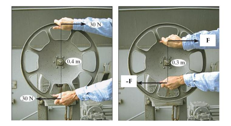
A torque or moment of 12 N·m is required to rotate the wheel. Would F be greater or less than 30 N?
