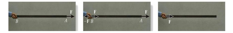
Moving a force from *A* to *B*, when both points are on the vector's line of action, does not change the **external effect**.
