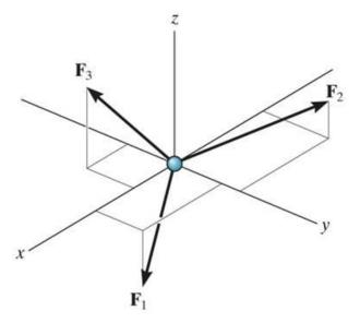
In contrast to the forces on a particle, the forces on a rigid-body are not usually concurrent and may cause rotation of the body. We can reduce the force and couple moment system acting on a body to an equivalent resultant force and a resultant couple moment at an arbitrary point O.
