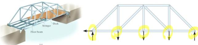
Load on deck transmitted to stringers, and from stringers to floor beams, and from floor beams to bridge trusses at joints.
