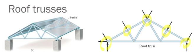
Load on roof transmitted to purlins, and from purlins to roof trusses at joints.
