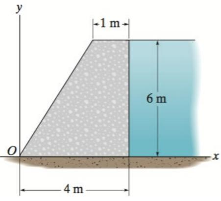
Determine the magnitude of the resultant force acting on the 100-m wide dam due to hydrostatic pressure. Let d = 2.5 m.
