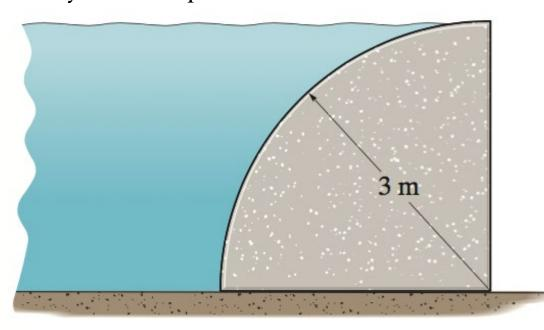
Determine the magnitude of the resultant force acting on gate *ABC* due to hydrostatic pressure. The gate has a width of 1.5 m.
