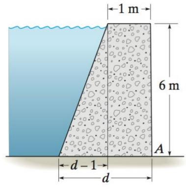
Determine the magnitude of the resultant force acting on on the 10-m wide dam due to hydrostatic pressure.
