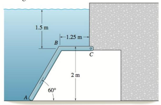
What is the *vertical* component of the resultant force acting on gate *ABC* due to hydrostatic pressure. The gate has a width of 1.5 m.
