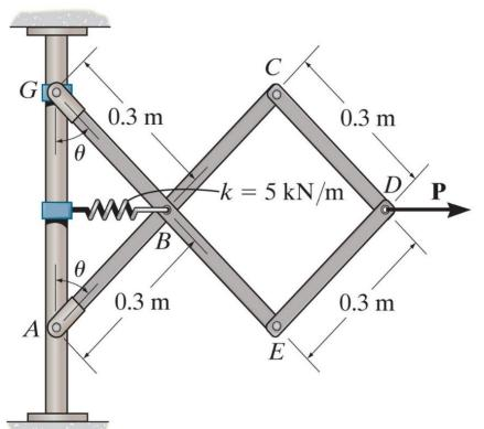
Determine the required force P needed to maintain equilibrium of the scissors linkage when the angle is 60 degrees. The spring is unstretched when the angle is 30 degrees.
