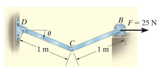
Determine the angle for F = 25 N equilibrium of the two-member linkage. Each member has a mass of 10 kg.
