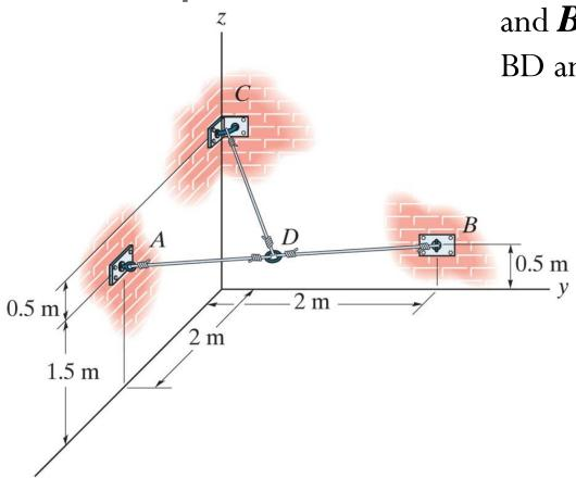
The ring at D is midway between points  $\boldsymbol{A}$  and  $\boldsymbol{B}$ . Determine the lengths of wires AD, BD and CD
