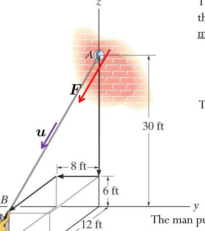
The force vector  $\mathbf{F}$  acting a long the rope can be defined by the unit vector  $\mathbf{u}$  (defined the <u>direction</u> of the rope) and the <u>magnitude</u> of the force.
