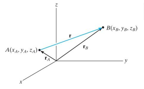
Thus, the (i, j, k) components of the positon vector r may be formed by taking the coordinates of the tail (point A) and subtracting them from the corresponding coordinates of the head (point B).
