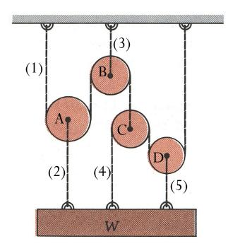
The five ropes can each take 1500 N without breaking. How heavy can *W* be without breaking any?
