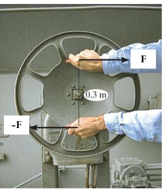
A torque or moment of 12 N·m is required to rotate the wheel.
