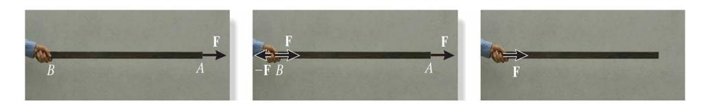
Moving a force from A to B, when both points are on the vector's line of action, does not change the **external effect**.
