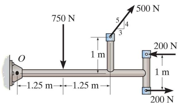
Replace the forces and couple system acting on the member by an equivalent force and couple moment acting at point O.
