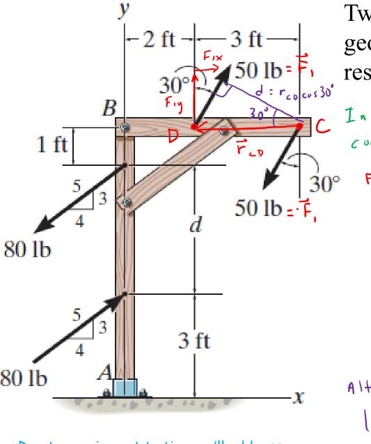
Due to running out to time, we'll address the typed problem statement in our next lecture. Hint to find  $M_R$ , need to also determine  $M_{lower}$ , such that  $M_R = M_{upper} + M_{lower}$  Two couples act on the beam with the geometry shown and d = 4 ft. Find the resultant couple
