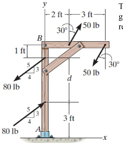
Two couples act on the beam with the geometry shown and d = 4 ft. Find the resultant couple
