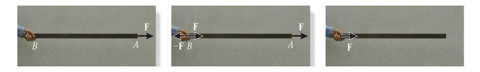
Moving a force from A to B, when both points are on the vector's line of action, does not change the **external effect**.
