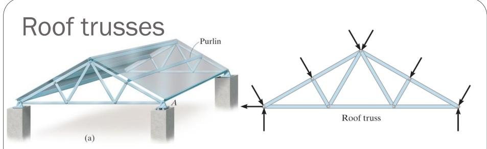
Load on roof transmitted to purlins, and from purlins to roof trusses at joints.
