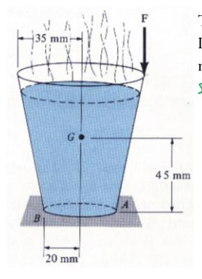
The cup is filled with 125 g of liquid. The mass center is located at G. If a vertical force F is applied to the rim of the cup, determine its magnitude so the cup is on the verge of tipping over.
