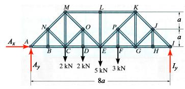
$$\begin{split} \Sigma F_x &= 0: & A_x &= 0 \,, \\ \Sigma F_y &= 0: & A_y + I_y - 2 - 2 - 5 - 3 &= 0 \,, \\ \Sigma M_A &= 0: & -2a(2) - 3a(2) - 4a(5) - 5a(3) + 8aI_y &= 0 \,. \\ \hline A_x &= 0, & A_y &= 6.375 \, \text{kN}, & I_y &= 5.625 \, \text{kN}. \end{split}$$
