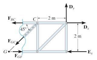
Determine the force in member GC of the truss and state if the member is in tension or compression.
