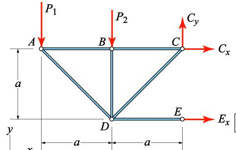
Next, start with a joint, draw the FBD, set it into *force* equilibrium *only*, and move to the next joint. Start with joints with at least 1 known force and 1-2 unknown forces.
