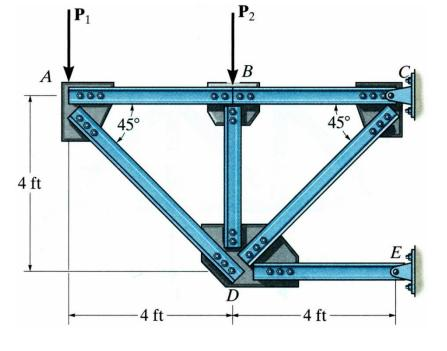
The truss, used to support a balcony, is subjected to the loading shown. Approximate each joint as a pin and determine the force in each member. State whether the members are in tension or compression.
