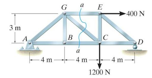
Determine the force in member GC of the truss and state if the member is in tension or compression.
