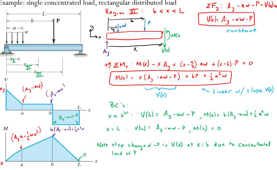
Explore and re-create the shear force and bending moment diagrams for the beam. Example: concentrated load, rectangular distributed load, concentrated couple moment
