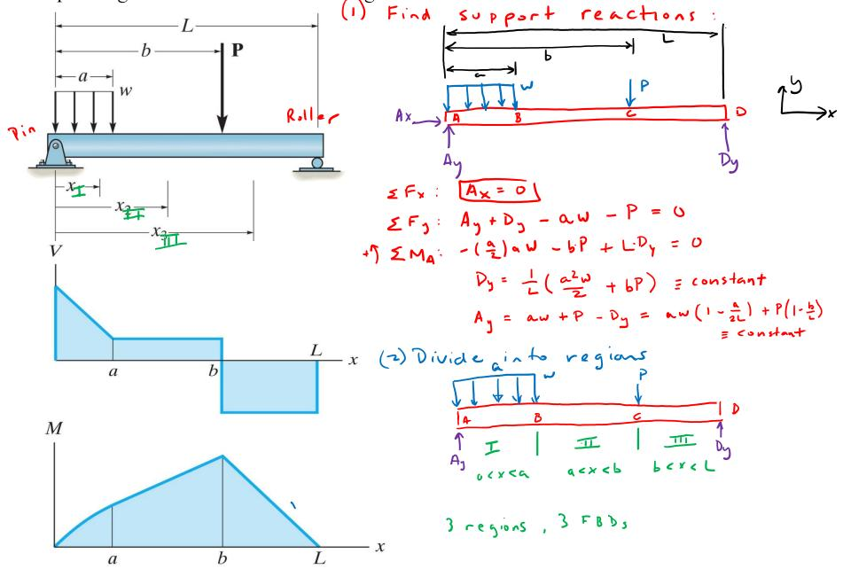
Explore and re-create the shear force and bending moment diagrams for the beam. Example: single concentrated load, rectangular distributed load  $\mathbf{z} = \mathbf{F}_{\mathbf{u}}$ :  $\mathbf{A}_{\mathbf{u}}$  -
