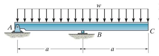
Draw the shear force and moment diagrams for the beam.
