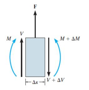
$$\Sigma F_y : \\ V + F - (V + \Delta V) = 0 \\ \Delta V = F \qquad \text{Jump in shear force due to} \\ \text{concentrated load } F$$
