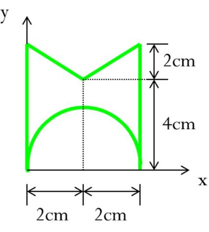
Locate the centroid of the cross section area.
