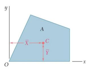
For example, the centroid of the area A is located at point C of coordinates  $\bar{x}$  and  $\bar{y}$ . In the case of a composite area, we divide the area A into parts  $A_1, A_2, A_3$
