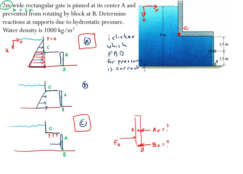
2m wide rectangular gate is pinned at its center A and prevented from rotating by block at B. Determine reactions at supports due to hydrostatic pressure. Water density is 1000 kg/m<sup>3</sup> W = Aron shape No "b" in this expression since b's cancel +) ZMB: -FR dR + Ax = = 0 => [Ax = 235.4 kN] EFx: F2-Ax-Bx=0
