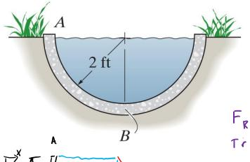
The semicircular drainage pipe is filled with water.
