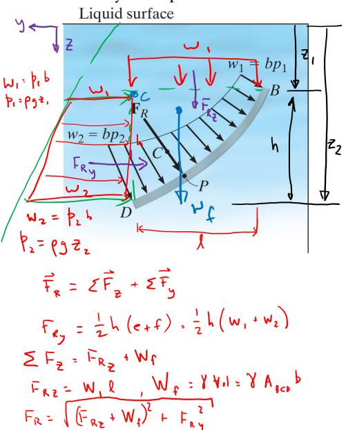
Determine the magnitude of the resultant hydrostatic force acting on the gate AB. The gate has width 1.5m.
