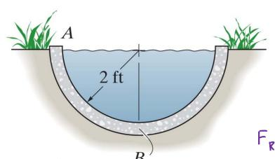
The semicircular drainage pipe is filled with water. Determine the resultant force that the water exerts on the side AB of the pipe per foot of pipe length. The specific weight of the water is  $\gamma = 62.4 \text{ lb/ft}^3$
