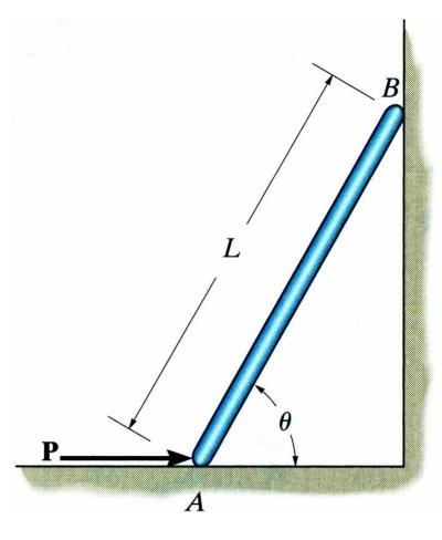
The thin rod of weight W rests against the smooth wall and floor. Determine the magnitude of force P needed to hold it in equilibrium.
