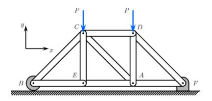
10) *Challenge*. Come up with your own truss and loading conditions that can be built with the kit and draw it in the space below. Determine which members are in tension and which members are in compression, then test your solution by building the truss.
