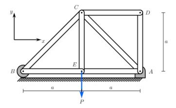
9) Determine which members in the truss below are in tension and compression, and check your solution by constructing the truss and apply appropriate loadings.
