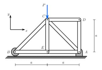
2) Use the FBD from Question 1 to find the support reaction forces at A and B in terms of the load P and distance a.
