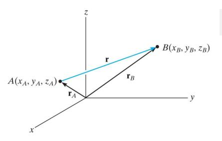
Thus, the (*i*, *j*, *k*) components of the positon vector *r* may be formed by taking the coordinates of the tail (point A) and subtracting them from the corresponding coordinates of the head (point B).
