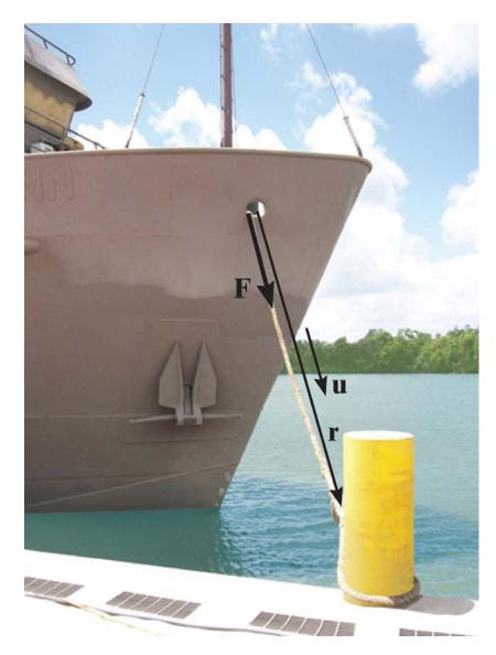
The force vector  $\boldsymbol{F}$  acting a long the rope can be defined by the unit vector  $\boldsymbol{u}$  (defined the <u>direction</u> of the rope) and the <u>magnitude</u>  $\boldsymbol{F}$  of the force.
