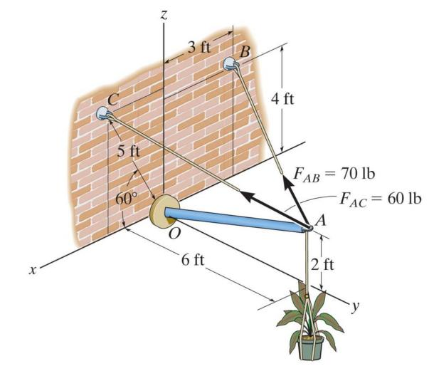
Determine the projected component of the force vector  $F_{AC}$  along the axis of strut AO. Express your result as a Cartesian vector
