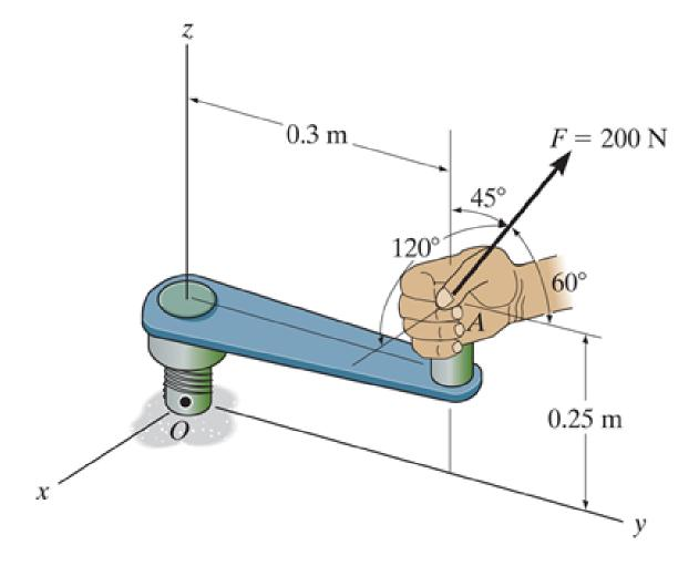
A force is applied to the tool as shown. Find the magnitude of the moment of this force about the x axis.
