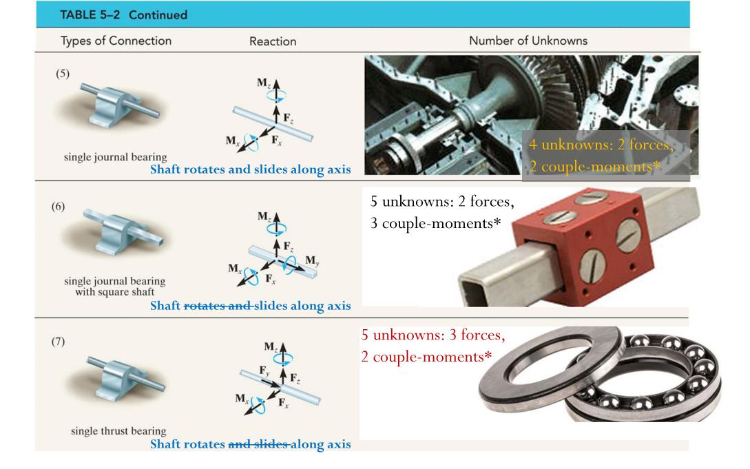
\* Couple-moments are not applied to FBD if the body is supported elsewhere by additional bearings, pins or hinges that are **properly aligned** to prevent rotation in one or more axes).
