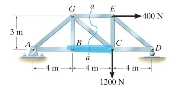
Determine the force in member BC of the truss and state if the member is in tension or compression.
