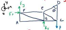
$$F_{y} = \left(1 - \frac{r_{AC}}{r_{FE}}\right) P$$
