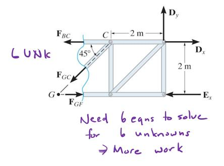
Determine the force in member BC of the truss and state if the member is in tension or compression.
