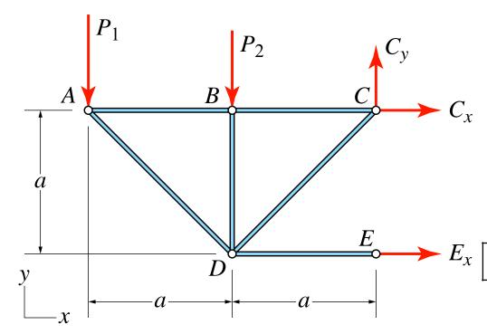
The truss, used to support a balcony, is subjected to the loading shown. Approximate each joint as a pin and determine the force in each member. State whether the members are in tension or compression.
