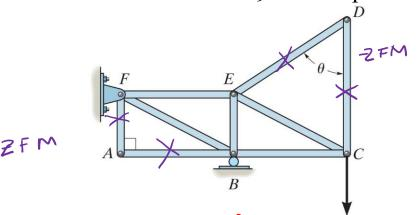
1) Solve for reaction forces by P considering the entire structure as one single rigid body.
