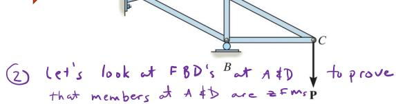
Assume that there are forces pointing in tension and aligned in direction of truss link members. Label forces as Fij where i is tail and j is acrow head
