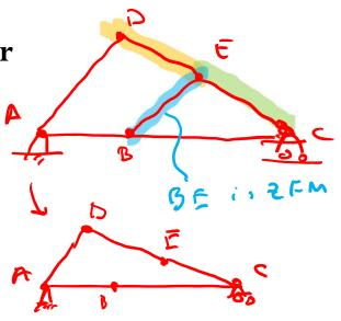
RECAP: Use Method of joints to prove that members attached to A and D should be FZM
