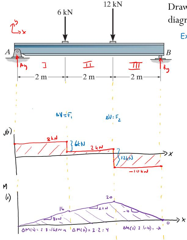
Draw the shear force and moment diagrams for the beam.
