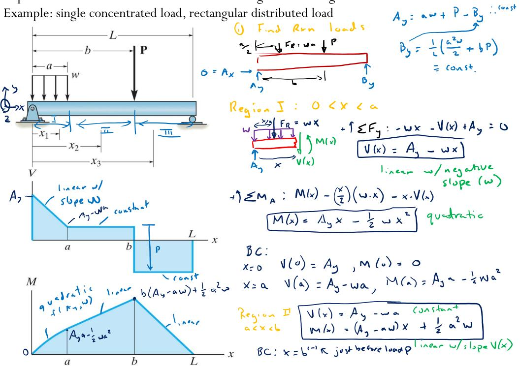
Explore and re-create the shear force and bending moment diagrams for the beam. Example: single concentrated load, rectangular distributed load
