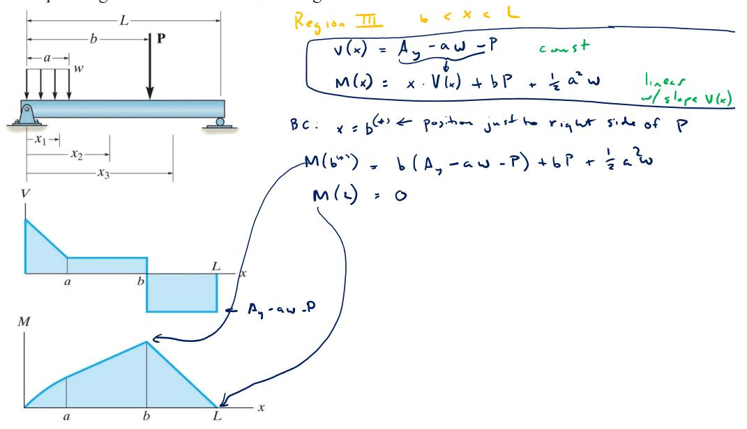
Explore and re-create the shear force and bending moment diagrams for the beam. Example: concentrated load, rectangular distributed load, concentrated couple moment
