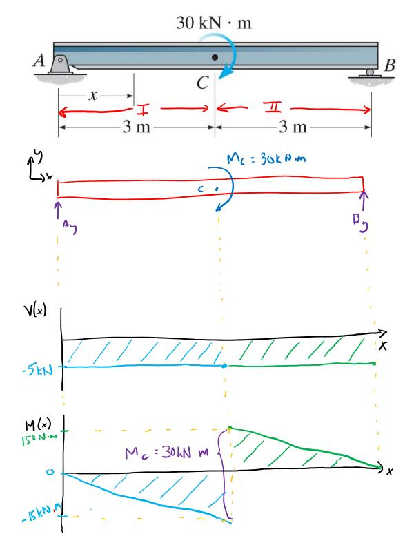
Draw the shear force and moment diagrams for the beam.
