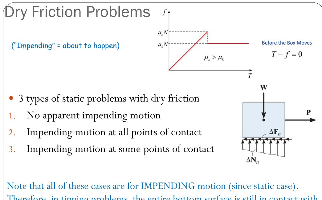
Note that all of these cases are for IMPENDING motion (since static case). Therefore, in tipping problems, the entire bottom surface is still in contact with ground.
