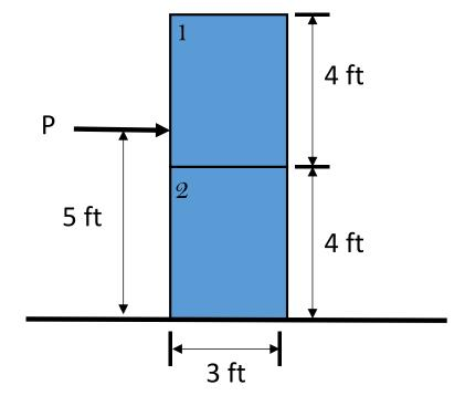
Two uniform boxes, each with weight 200 lb, are simply stacked as shown. If the coefficient of static friction between the boxes is  $\mu_s = 0.8$  and between the box and the floor is  $\mu_s = 0.5$ , determine the minimum force *P* to cause motion.
