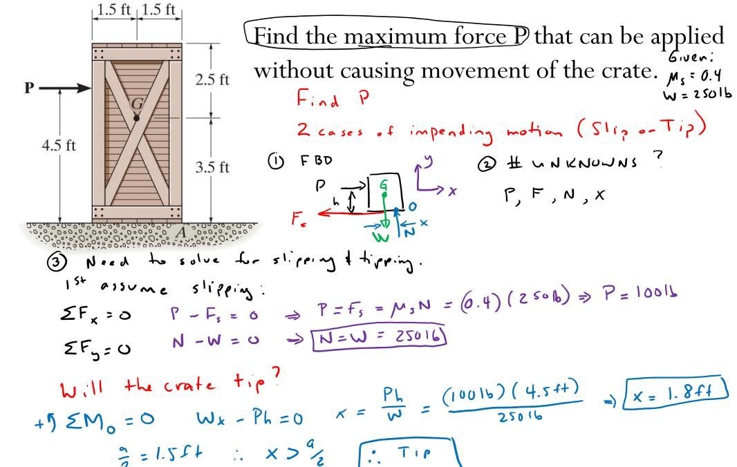
Must solve for P that causes initial tipping (551) (250 1%)  $\sum M_0 = 0 \rightarrow M \times Ph = 0 \Rightarrow P = \frac{1}{L} = \frac{4.5 \text{ ft}}{4.5 \text{ ft}}$   $\therefore P = 83.3 \text{ lb } | Finally$
