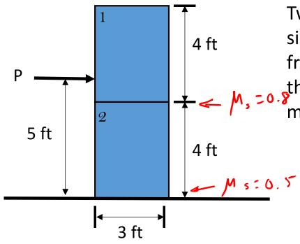
Two uniform boxes, each with weight 200 lb, are simply stacked as shown. If the coefficient of static friction between the boxes is  $\mu_s=0.8$  and between the box and the floor is  $\mu_s=0.5$ , determine the minimum force P to cause motion.
