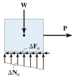
Note that all of these cases are for IMPENDING motion (since static case). Therefore, in tipping problems, the entire bottom surface is still in contact with ground.
