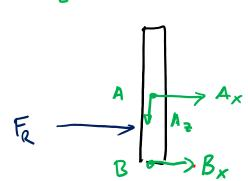
2m wide rectangular gate is pinned at its center A and prevented from rotating by block at B. Determine reactions at supports due to hydrostatic pressure. Water density is 1000 kg/m<sup>3</sup>
