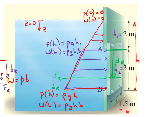
2m wide rectangular gate is pinned at its center A and prevented from rotating by block at B. Determine reactions at supports due to hydrostatic pressure. Water density is  $1000 \text{ kg/m}^3$
