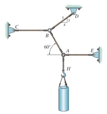
**Problem 3:** Given the mass of the crate is m, perform equilibrium analysis on point A to determine the tension developed in the cables AB.
