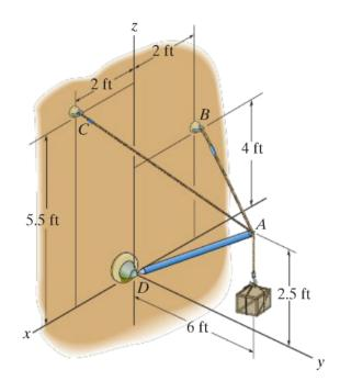
**Problem 4:** A traffic light with weight W is supported by three cables as shown. Perform equilibrium analysis on point A to determine the tension in each wire. Include the unit vectors what give the directions of the forces acting on point A.
