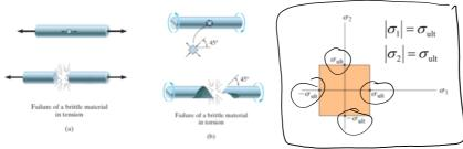
Due to material imperfections, tensile fracture of a brittle material is difficult to predict, and so
