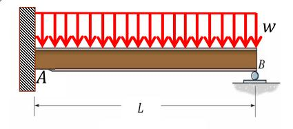
Obtain the reaction at the support B using
