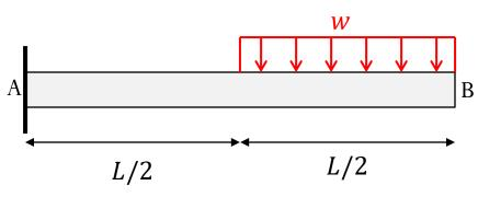
Find the deflection at point B at the end of the cantilever beam
