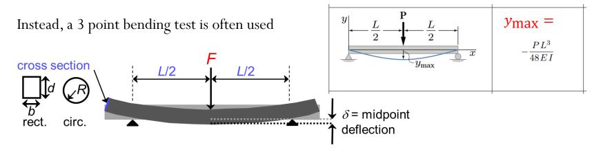
Find an expression for the stiffness E of the material, given the geometry, applied load F, and deflection  $\delta$  at the midpoint
