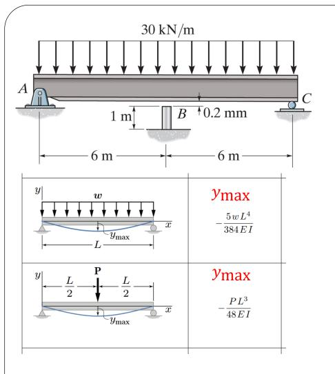
Before the uniform distributed load is applied on the beam, there is a small gap of 0.2 mm between the beam and the post at B. Determine the support reactions at A, B, and C. The post at B has a diameter of 40 mm, and the moment of inertia of the beam is  $I = 875 \times 10^6 \text{ mm}^4$ . The post and the beam are made of material having a modulus of elasticity of E = 200 GPa.
