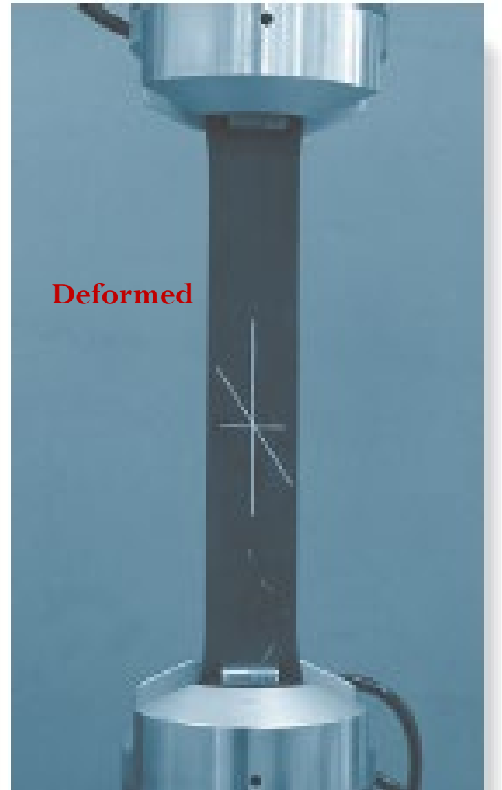
Rubber membrane subject to tension
