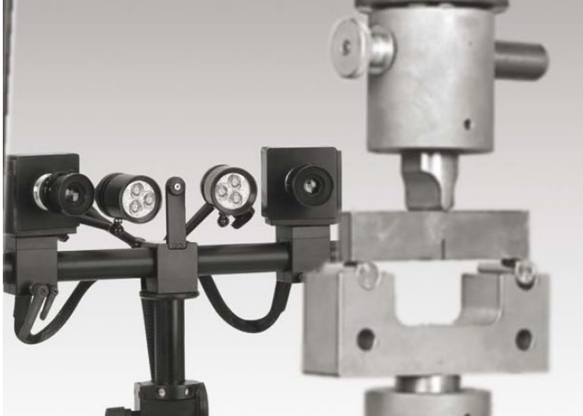
DIC system analyzing a notch fracture test, from trillion.com
