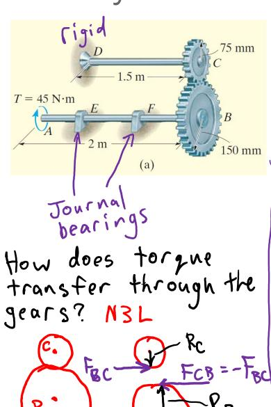
Two solid steel shafts are connected through gears at points B and C. The top shaft is mounted to a fixed wall at point D. Determine the angle of twist at point A assuming a torque of  $T = 45 \text{ N} \cdot \text{m}$  is applied at A. Each shaft has a diameter of d = 20 mm and a shear modulus of G = 80 GPa
