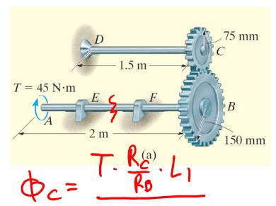
Two solid steel shafts are connected through gears at points B and C. The top shaft is mounted to a fixed wall at point D. Determine the angle of twist at point A assuming a torque of  $T = 45 \text{ N} \cdot \text{m}$  is applied at A. Each shaft has a diameter of d = 20 mm and a
