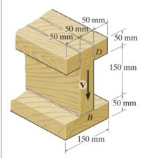
A beam is made of four planks glued together. Knowing that the vertical shear in the beam is  $V=500~\rm N$ , determine the minimum required shear strength  $\tau_g$  for the glue.
