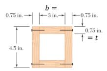
A square box beam is constructed from four planks as shown. Knowing that the spacing between nails is 1.5 in. and the beam is subjected to a vertical shear of magnitude V = 600 lb, determine the shearing force in each nail.
